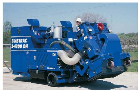
*The front end lift system raises the blast head for transport*
